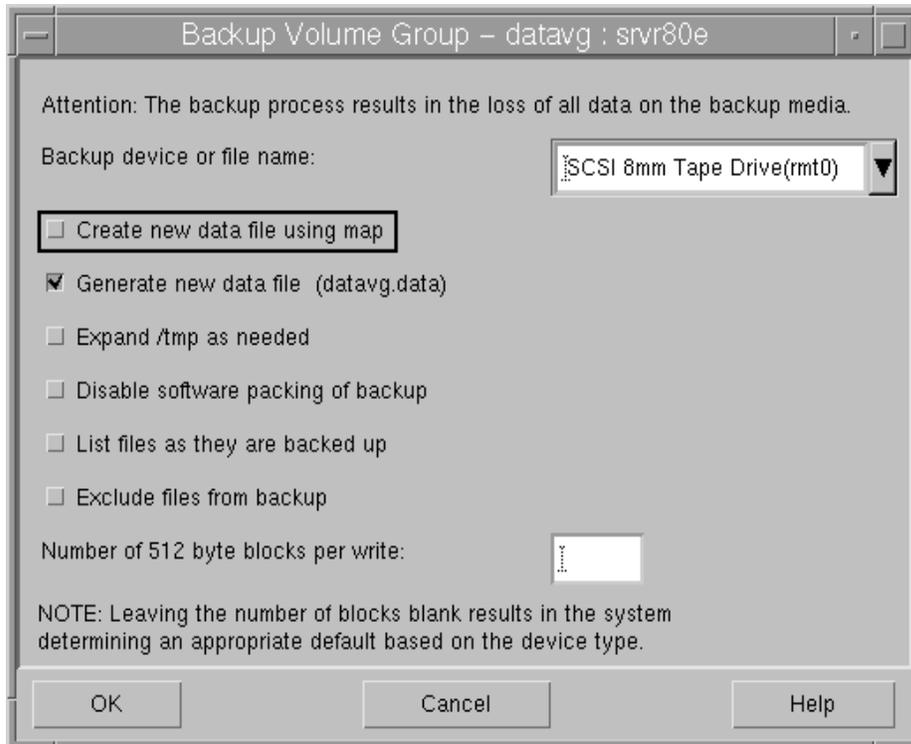
Figure 4-6 Backup of a non-root volume group with Web-based System Manager
