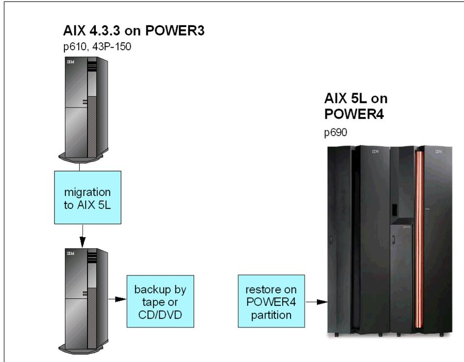
Figure 4-2 Migration of AIX 4.3 POWER3 machine to AIX 5L POWER4 partition
