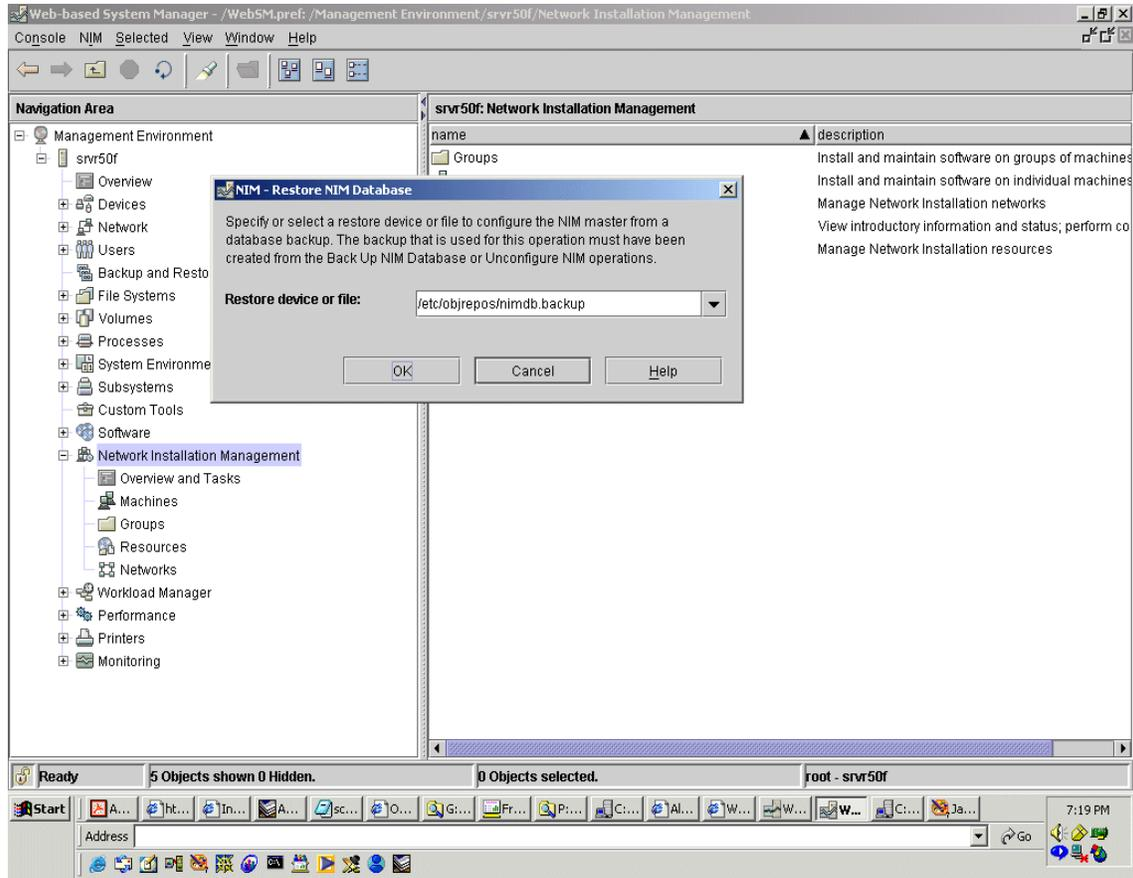
Figure 6-5 Restore of NIM database using the Web-based System Manager
