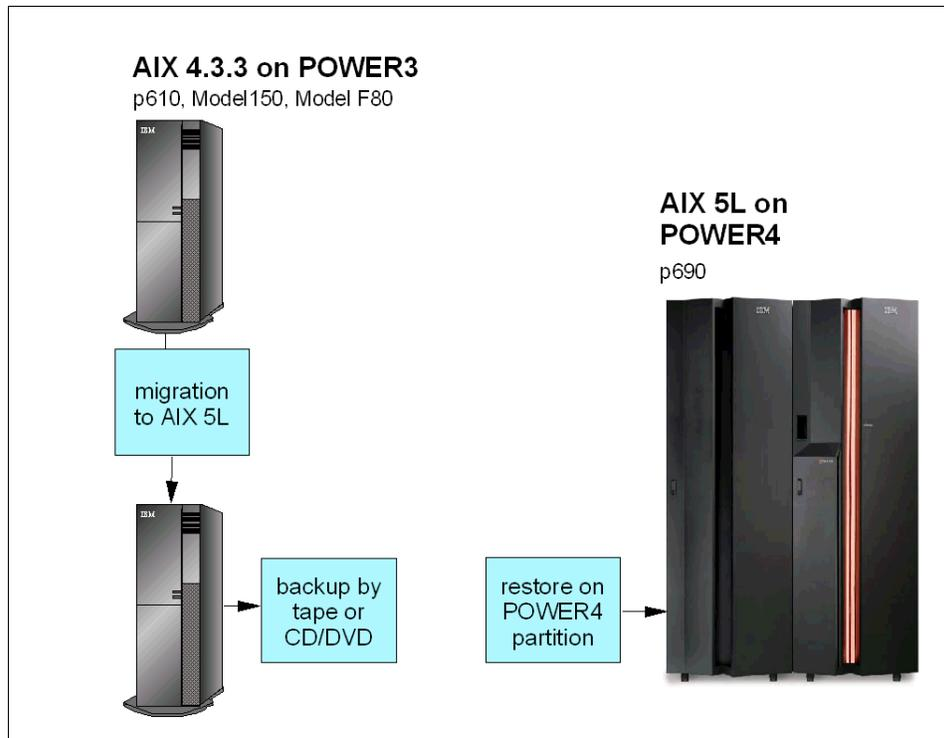
Figure 5-1 Migration of POWER3 machine to AIX 5L POWER4 partition
