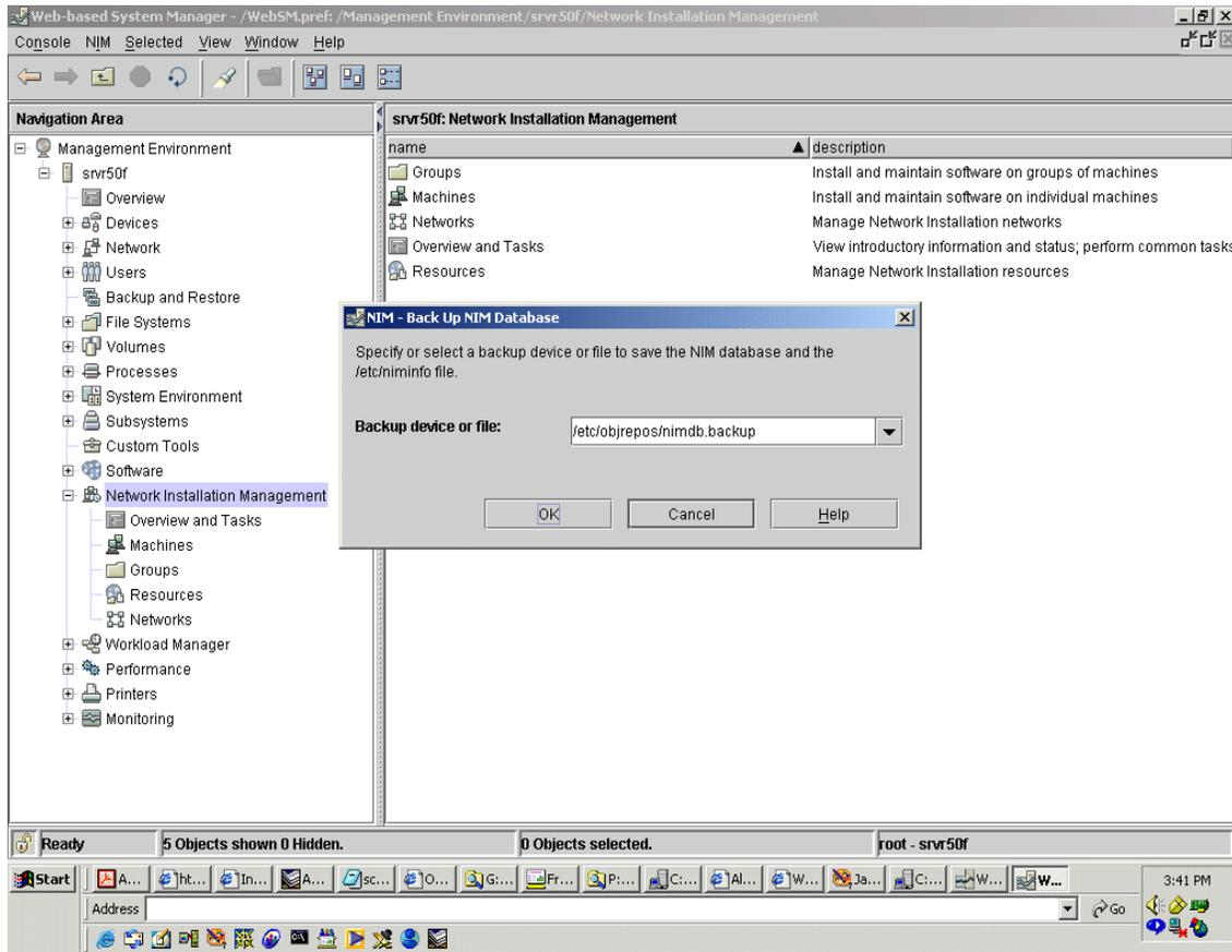
Figure 6-3 Creating a NIM database backup using Web-based System Manager
