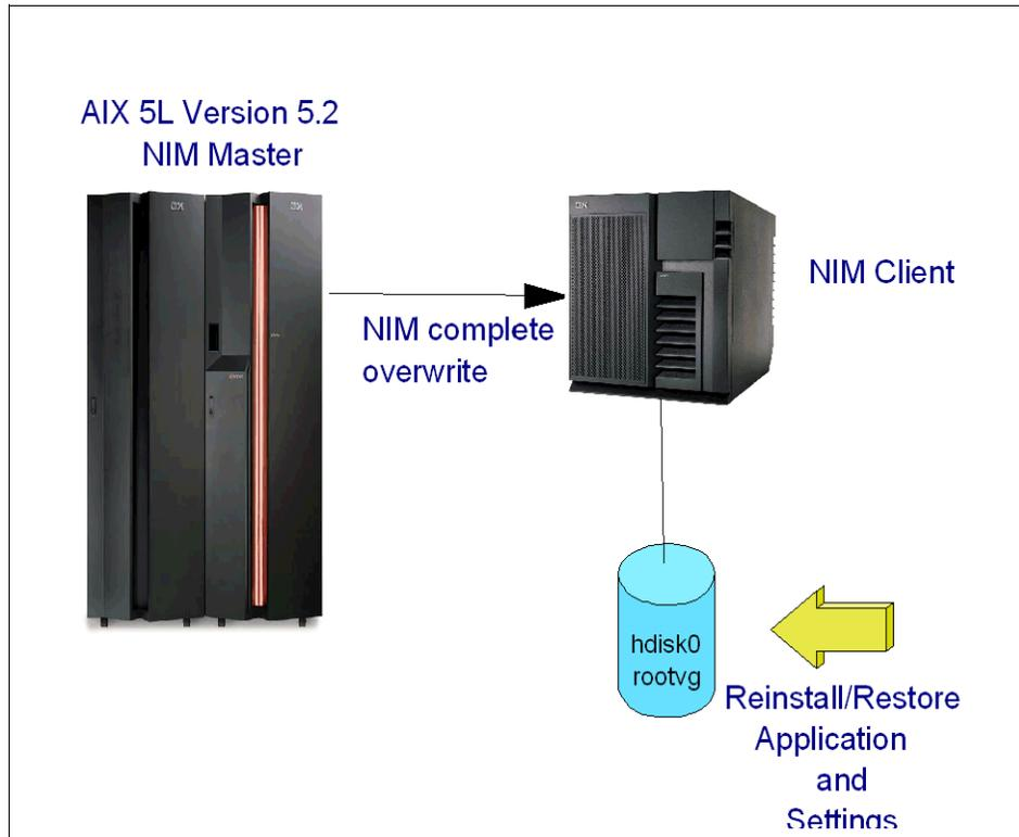
Figure 6-8 New installation of AIX 5L Version 5.2 over the network
