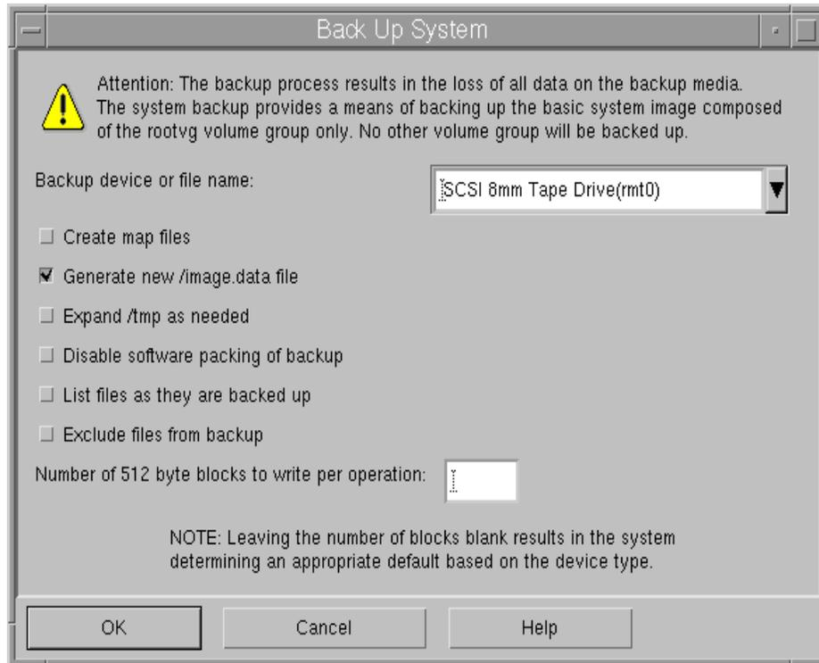
Figure 4-5 Backup menu using the Web-based System Manager
