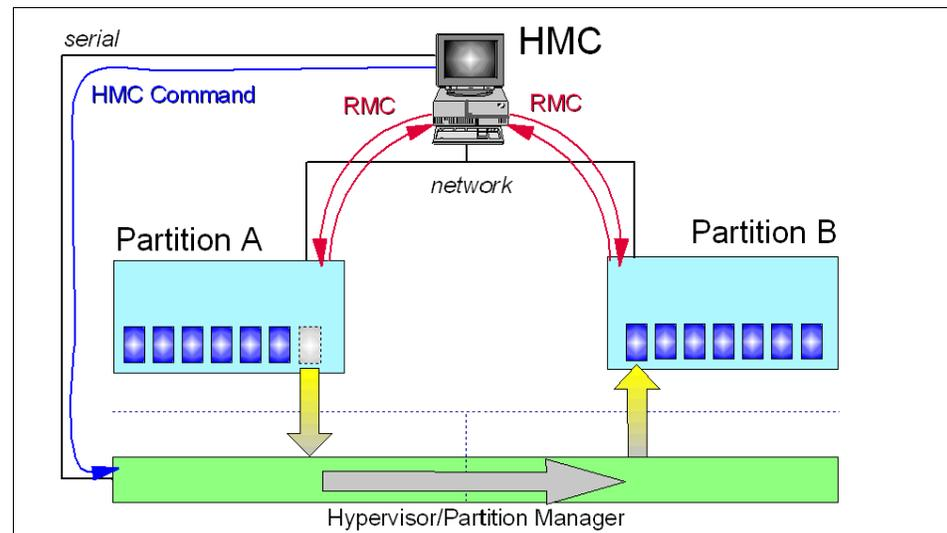
Figure 2-1 Concept of Dynamic Logical Partitioning (DLPAR)
