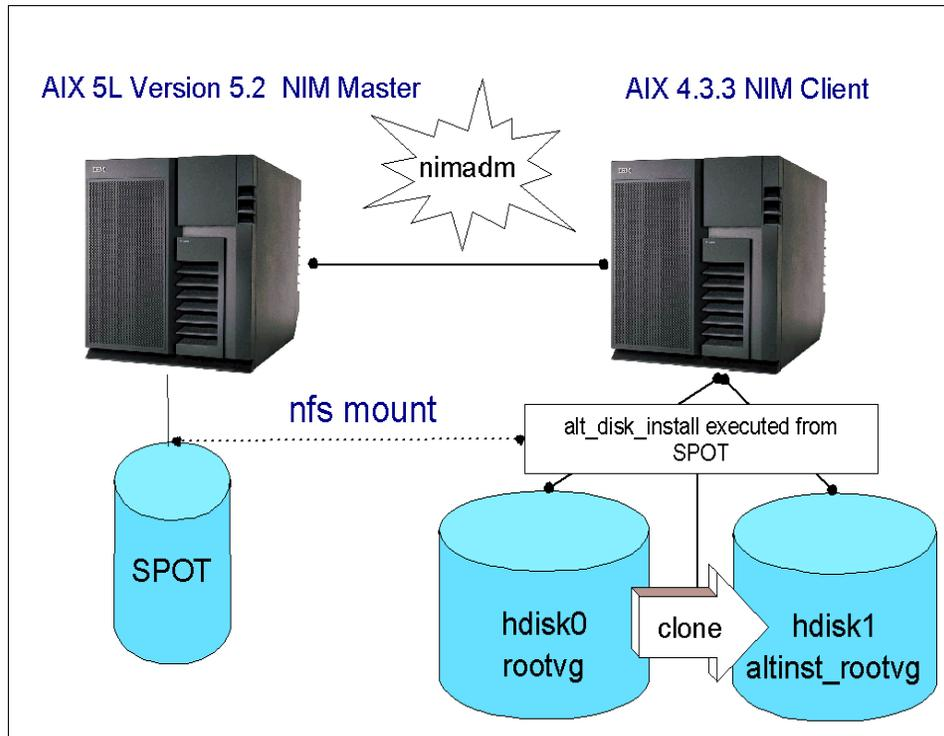
Figure 6-9 Alternate disk migration: The cloning process
