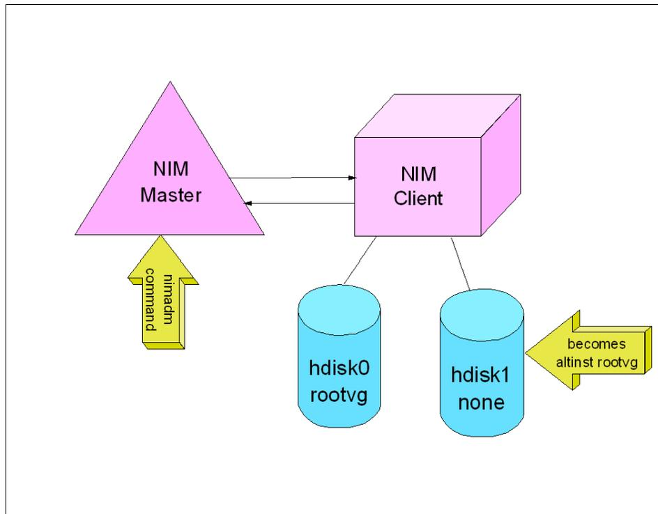
Figure 6-1 Graphical overview of alternate disk migration concept
