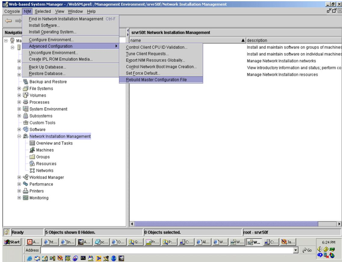
Figure 7-2 Rebuilding `/etc/niminfo` file using the Web-based System Manager
